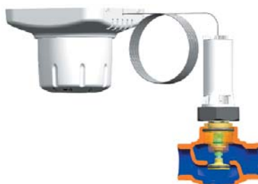
Room temperature above the target value, valve opened
