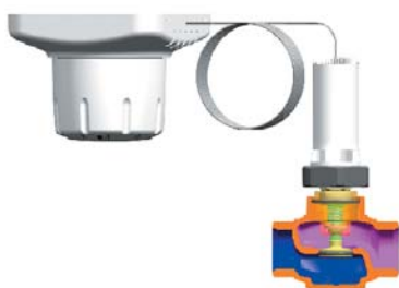
Room temperature under the target value, valve closed
